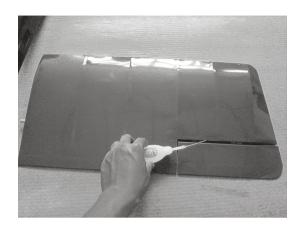
1.Allow enough hinge gap to ensure maximum control throws. Next, place 3-4 drops of thin CA to both side of all hinges. Do not over soak the CA hinges. Glue may run out and cause binding. We recommend using a clear covering to seal the gaps on all control surfaces
