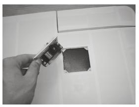
3. Secure the servo plug to the wing with tape to keep it from slipping inside the wing.
