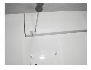
Use two 2mm x 25 mm bolts to mount control horn.
