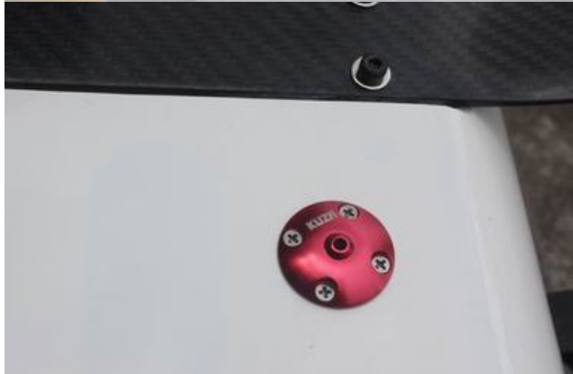
Aluminium Backplate Hollowed-out Electric Spinner included for electric power(Excellent cooling effect for brushless motor)
