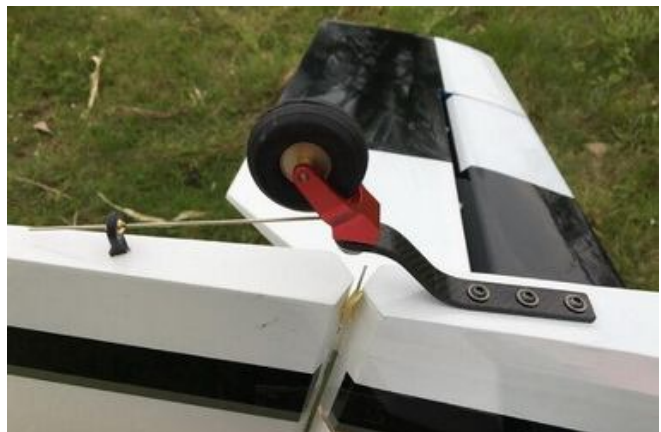
KUZA V2 version Carbon fiber tail wheel assembly with CNC machined metal parts, including the aluminium tail wheel hub.
