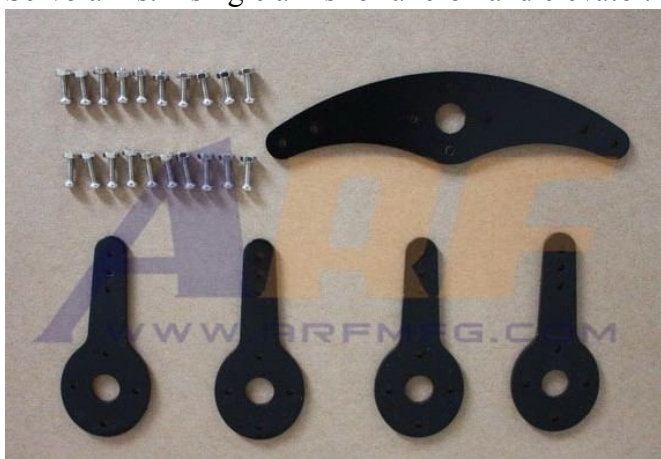
Servo arms: 4 single arms for aileron and elevator. 1 dual arm for rudder.
